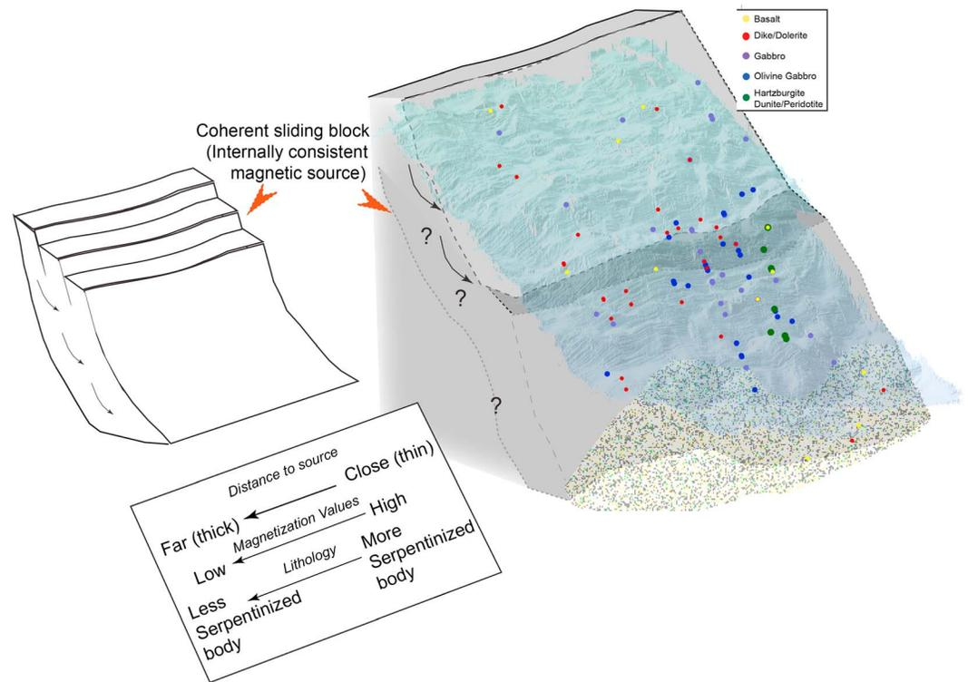
**Figure 7.** A schematic summary of magnetic sources of the Hess Deep south facing slope, with microbathymetry with color coded sample locations overlying the inferred slipped surface and the middle slope bench of Ferrini *et al.* [2013].
