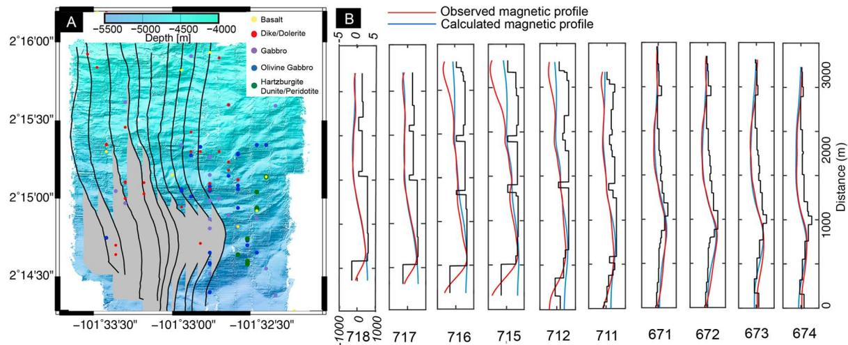
**Figure 4.** (a) Observed magnetic anomalies over the south facing slope of Hess Deep. (b) Track-by-track forward modeling results. The red and blue solid lines indicate modeled and observed anomalies, respectively. The black solid lines indicate the final intensity of magnetization for the block models (A/m). See the detailed calculation method in section 3.4.2.
