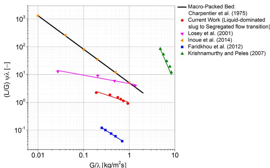
**Fig. 6.** Flow map comparison of a conventional trickle bed reactor: Charpentier and Favier (1975) and micro-packed reactors: Faridkhou and Larachi (2012), Losey et al.
