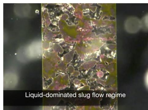
**Video 1.** Optical microscope observation of the hydrodynamics during liquid-dominated flow regime,  $u_L=9.3 \times 10^{-4}$  m/s,  $u_G=0.31$  m/s. Supplementary material related to this article can be found online at <http://dx.doi.org/10.1016/j.ces.2016.03.018>.
