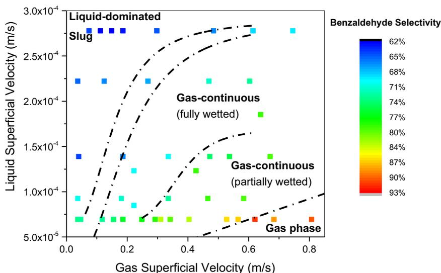
Fig. 10. Benzaldehyde selectivity colour-mapped dot plot superimposed on the flow regime map.
