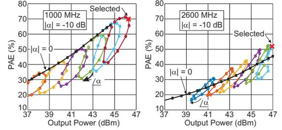
Fig. 7. Measured PAE vs. Output power, with  $X$  at open circuit. With no CSP (black squares) and with  $|\alpha|$  @ -10 dB, with 30 degree phase steps (colored circles), at different input power levels.
