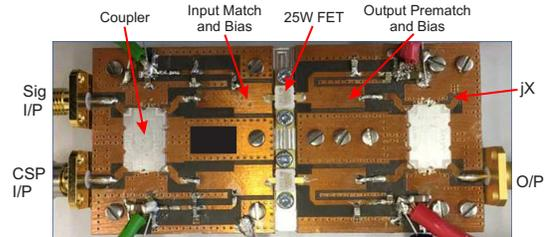
Fig. 4. Demonstrator board picture. (Size: 86 mm  $\times$  42 mm).
