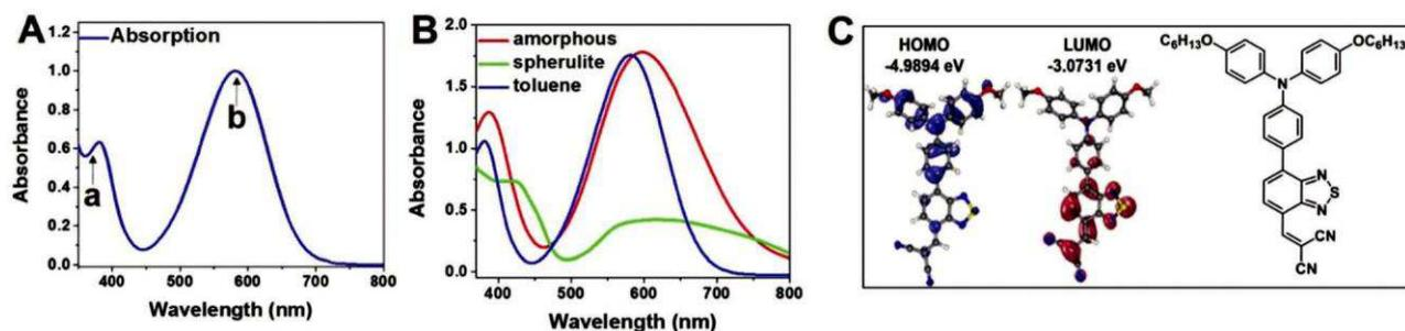
Fig. 1 (A) Absorption spectrum of C6-TPA-BT-CN in toluene: (a) 381 nm, (b) 581 nm. (B) Absorption spectra of C6-TPA-BT-CN in toluene (blue), amorphous film (red), and non-banded spherulite  $5 \text{ mg mL}^{-1}$  film (green). (C) Frontier molecular orbitals (HOMO and LUMO) calculated with B3LYP/6-31G\* Basis Set-Orca software, and molecular structure of C6-TPA-BT-CN.
