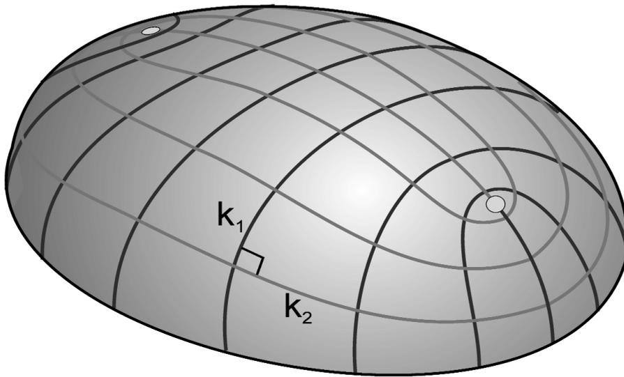
**Figure 3.** Ellipsoidal dome with lines of curvature and two umbilical points (modified from Hilbert and Cohn-Vossen, 1952).
