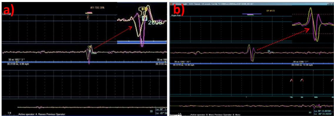
Fig. 5.7 Typical induced voltage signatures indicating the presence of transverse flaw probed with: a) longitudinal sensor SL (purple curve) and normal sensor SN (yellow curve); b) longitudinal sensor SL (purple curve) and tangential sensor ST (yellow curve).
