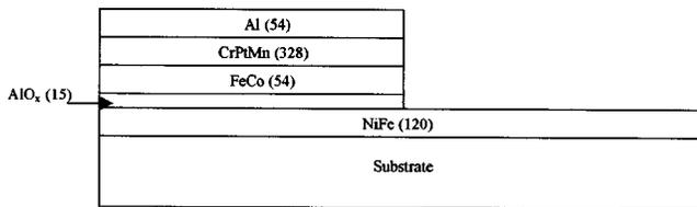
FIG. 1. Schematic diagram showing the multilayered structure of the magnetic tunnel junction sample (dimensions shown in angstroms).
