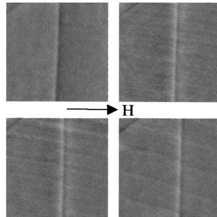
FIG. 3. Magnetic force images of junction and electrode at, from left to right and top to bottom, 100, 400, 200, and a return to 0 Oe. Images are also in chronological order.
