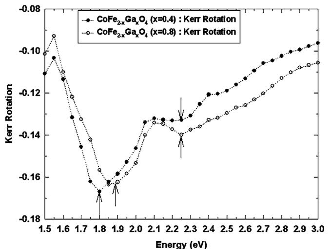
FIG. 3. Magneto-optic Kerr rotation spectra for  $\text{CoFe}_{2-x}\text{Ga}_x\text{O}_4$  ( $x=0.4$  and  $x=0.8$ ) samples.
