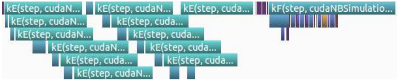
Figure 2. Visual profiling data for a move. Asynchronous execution of s streams where the total block and shared memory conditions are not met. Overlapping is divided into stream groups that meet the hardware's block and shared memory restrictions. The kE blocks represent the non-bonded energy kernels, and the corresponding ones under the kF block are the bonded forces and the 3D grid binning kernels.
