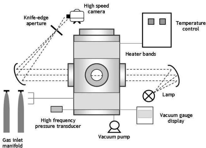
**Figure 2.1** Diagrammatic layout of CVCB with ancillary components
