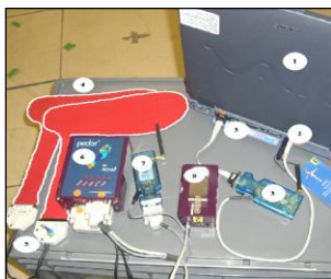
Fig 2: Pedar Equipment for data collection; includes laptop 1 , Pedar pen drive software 2 , blue-tooth adapter/receiver 3 , insoles 4 , double Pedar insole cable 5 , cable box receiver 6 , secondary blue-tooth adapter 7 , power supply 8
