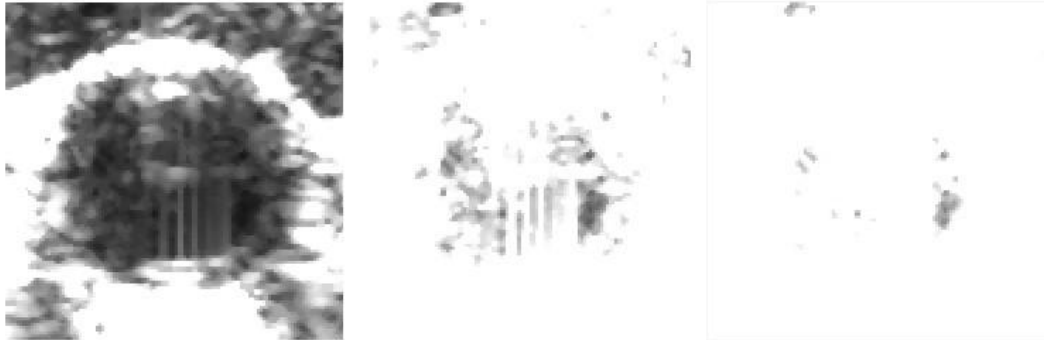
Figure 4.10: [Left] B-mode image with gain of 5; [Middle] Gain of 20; [Right] Gain of 50.
