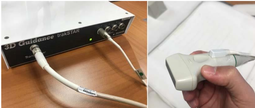
Figure 6.4: [Left] The trakstar base amplifier unit. [Right] The position sensor attached to the ultrasound linear probe with double-sided tape.
