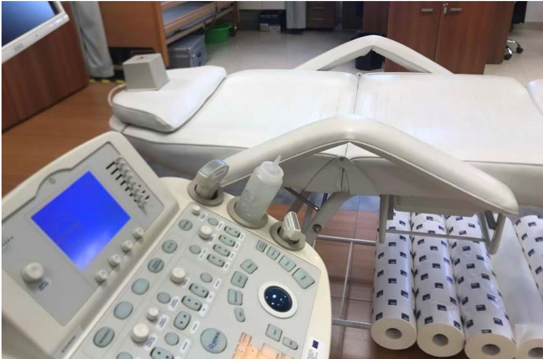
Figure 6.3: The electromagnetic transmitter is positioned at the head of the couch, closest to the imaging area as possible.
