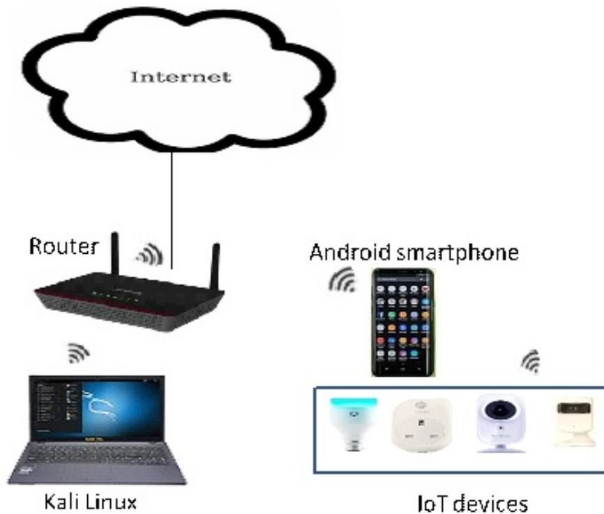
**Figure 3.3: Detecting the behavior of the IoT user testbed network architecture.**
