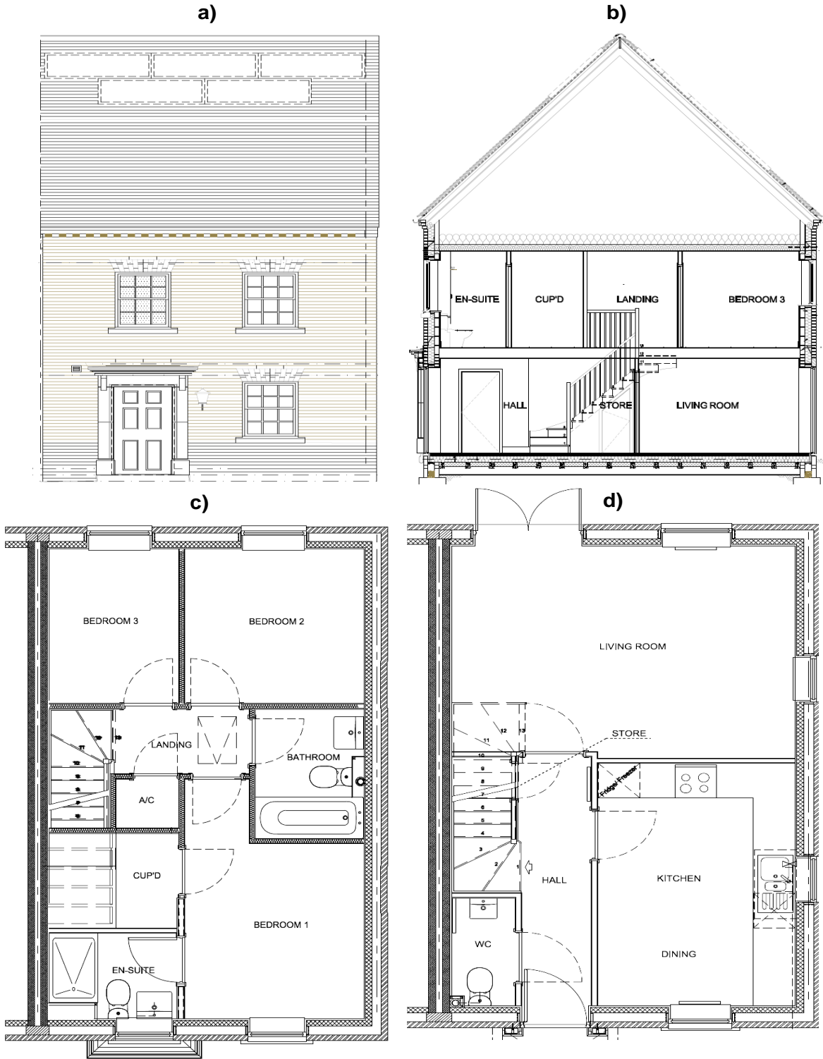
Figure 3-5: Domestic dwelling floorplan views with defined zones. a) front view; b) cross-section view; c) first floor plan view; and d) and ground floor plan view.
