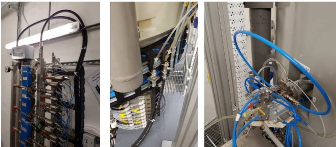
Figure 56 Modified water and He cooling of the COSTIS STS.
