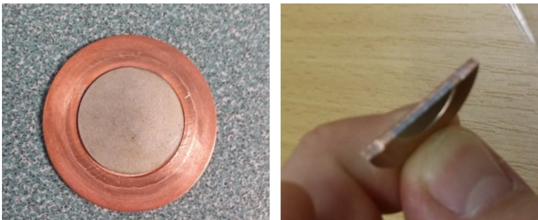
Figure 60 Mo targets sintered on Cu backing provided by TRIUMF.
