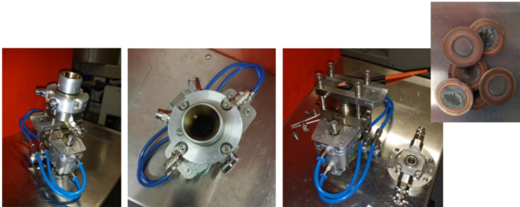
Figure 66 COSTIS STS and target discs after irradiations showing no visual evidence of damage
