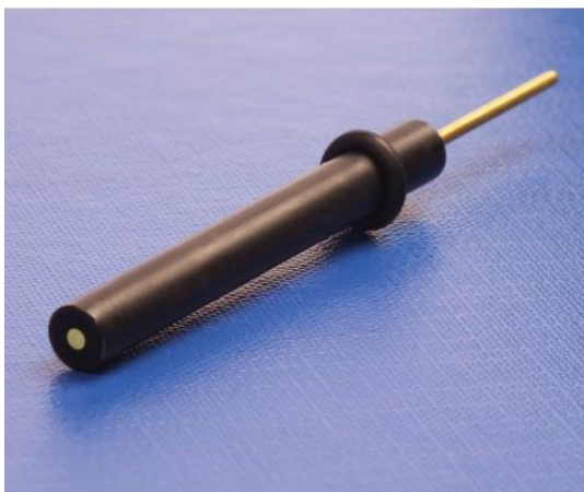
Figure 1.10: A working electrode with a 2mm diameter gold surface (108).
