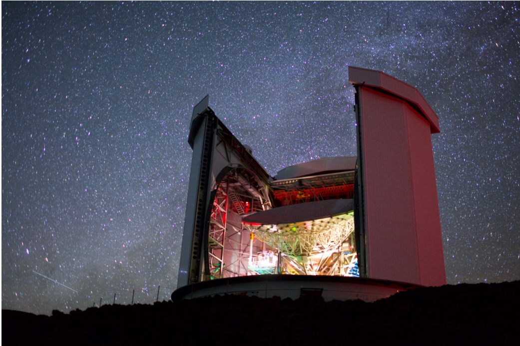
Figure 2.10. Image of the JCMT, showing the telescope dome and primary mirror. A Gore-Tex sheet can be manoeuvred in front of the mirror to allow for continuous day and night observations, while protecting the telescope from wind and particulate damage. Image credit East Asian Observatory (2017).
