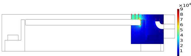
Fig. 7. Cross section of the parallel plate resonator. The color gradient show the electric field (V/m) at the edge of the reference plate. The geometry and placement of the capacitive coupling probe is also shown.
