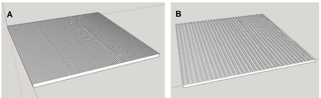
*Figure 7.* Schematic of tactile plates created using 3-D printer technology. (A) Tactile plate with high spatial frequency. (B) Tactile plate with low spatial frequency.
