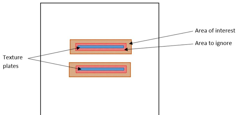
*Figure 9.* Schematic diagram showing an aerial view of the arena used in Experiment 1a tracked using Ethovision software. Tracking activity of interest (orange) and areas to ignore (red). Tactile plates are represented by the blue and are not to scale.
