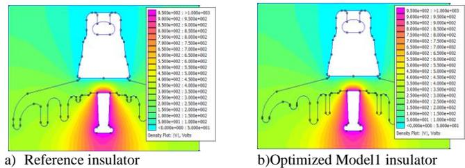
Figure 6. Equipotential distribution under clean surface conditions.
