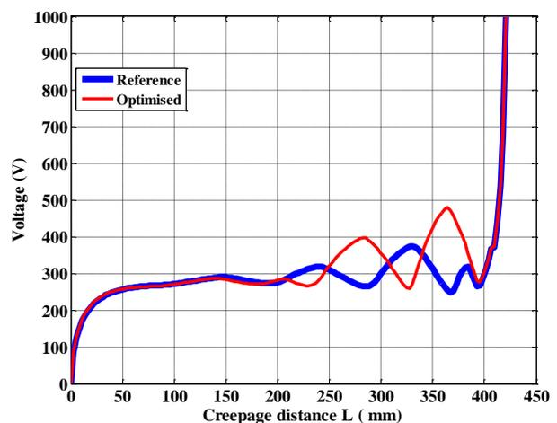
Figure 7. Potential distribution along the clean insulator profile for the standard and optimised Model 1 insulator shapes. (creepage path cap to pin)
