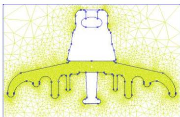
Figure 5. Meshed model used in Finite Element computations.
