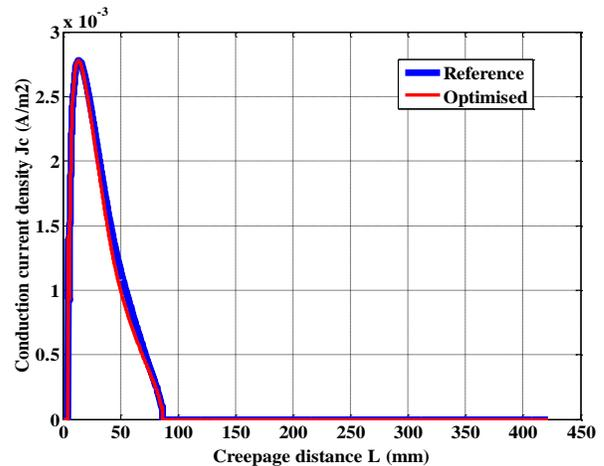
**Figure 18.** Conduction current density distribution along the creepage distance for Scenario 7 (pollution on upper surface  $S_1$ ).
