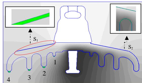
Figure 1. F12AS Type glass insulator depicting details of shape, pollution layer and water droplet formation on the ribs.
