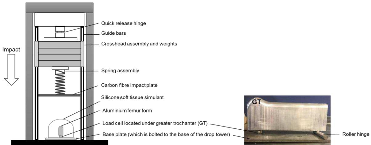
**Figure 1.** Schematic of the Instron Dynatup 9250-HV and the experimental setup for measuring the peak compressive force applied to the proximal femur during a simulated sideways fall from standing height (CSA EXP-08-17).
