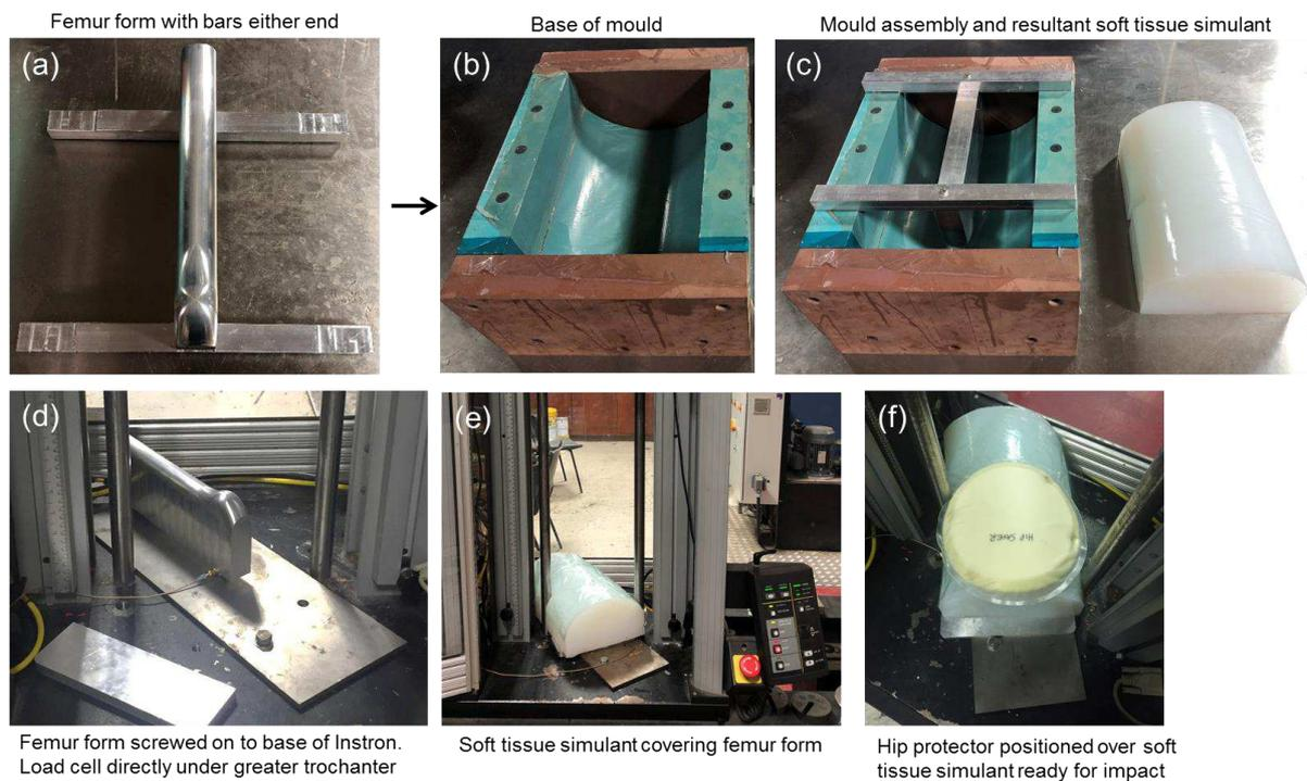
**Figure 2.** Two-part assembly casting mould for silicone soft tissue simulant with resultant cured silicone (a–c). Setup of femur form screwed on to base of drop tower with soft tissue silicone and hip protector (d–f).
