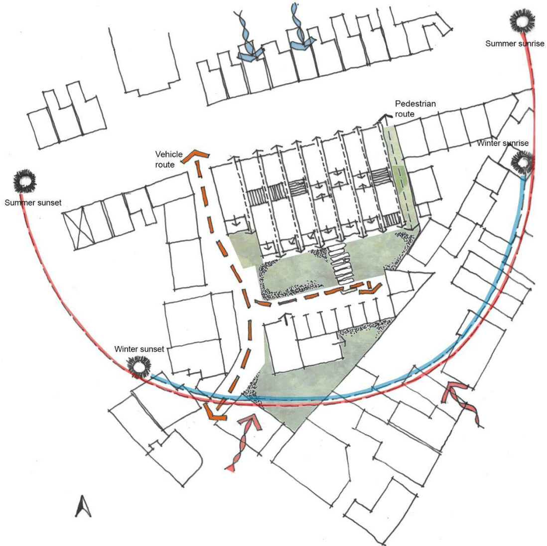
Figure 150: Siting and design concept. This drawing reveals the proposed arrangement of 12 dwellings on the site and the reason for such it. By placing 8 terrace houses along the street frontage of New Road may restore the continuity of the street, therefore contribute to the reinforcement of the boundary. Geographic conditions are also considered at this stage to benefit the passive design afterwards.
