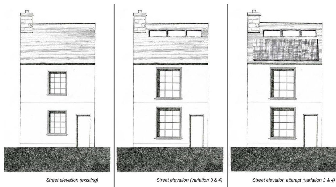
Figure 132: Changes of building's street frontage façade: from left to right, under strict conservation, less conservation, the elevation possibly jeopardise streetscape.
