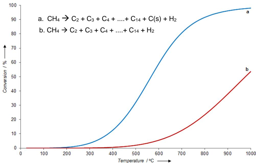
**Figure S2:** Thermodynamic CH<sub>4</sub> conversion against temperature (a) with coke formation allowed, (b) without coke formation allowed (calculated using HSC Chemistry 8.6)
