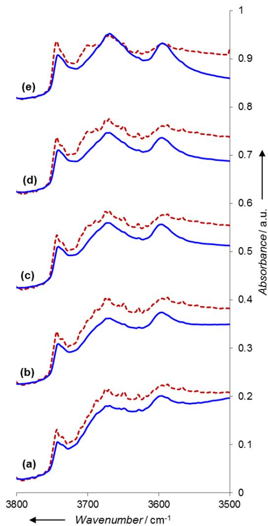
**Figure S4:** IR spectra for hydroxyl group region for H-ZSM-5 (dotted) and ABZ-5 (undotted), (a) at 25 °C, (b) at 100 °C, (c) at 200 °C, (d) at 300 °C, (e) at 400 °C
