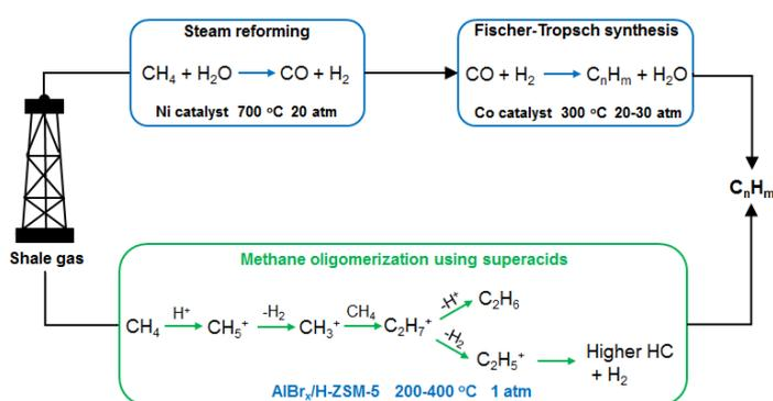
**Figure 1.** Current and proposed process for converting methane into olefins and fuels. At present, methane is reformed into syngas and then transformed into higher hydrocarbons through the Fischer-Tropsch synthesis. This indirect process requires high temperatures and pressures. Methane oligomerization using solid superacids offers a direct route to converting methane into higher hydrocarbons under mild conditions.
