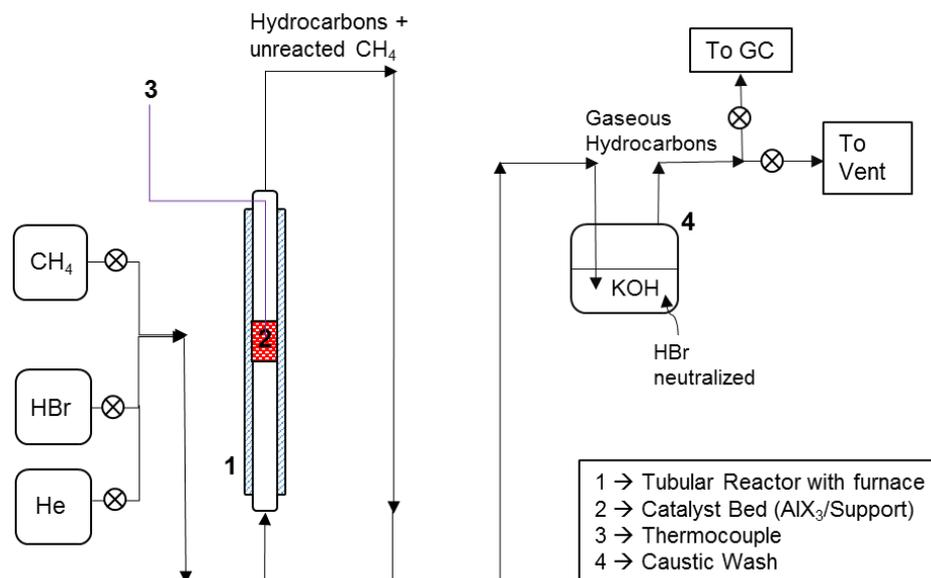
Figure S1: Schematic for CH<sub>4</sub> reaction system
