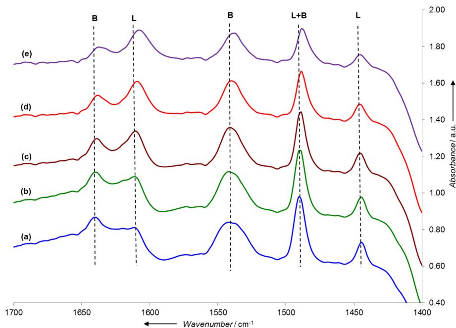
**Figure S6:** DRIFTS spectra for SZ catalysts after pyridine desorption at (a) 25 °C, (b) 100 °C, (c) 200 °C, (d) 300 °C, (e) 400 °C
