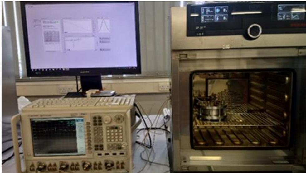
Figure 6-3 Photograph of the bench-top experimental assembly for cavity measurements. The cavity is put inside a computer-controlled oven and connected to a network analyser under control of a LabVIEW program.
