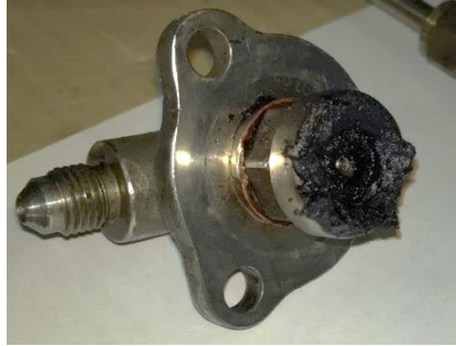
Figure 9: Fuel nozzle coking.
