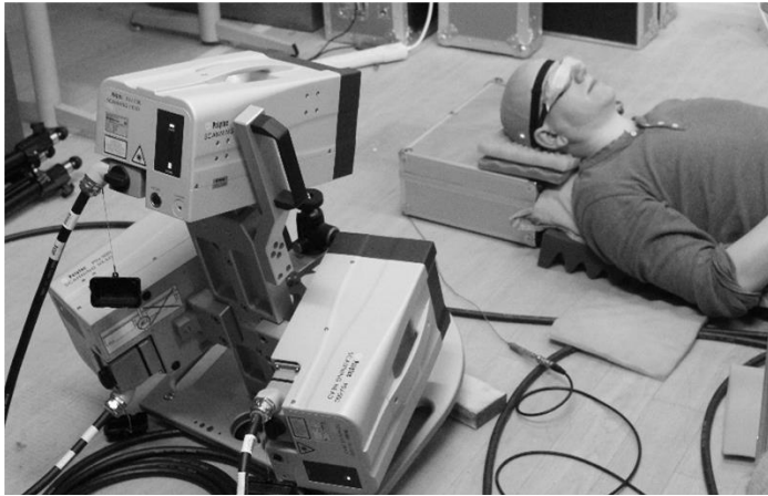
Figure 1 Three Polytec™ PSV-500 vibrometers focusing on participants right temporoparietal region (contralateral to the B71 bone transducer).
