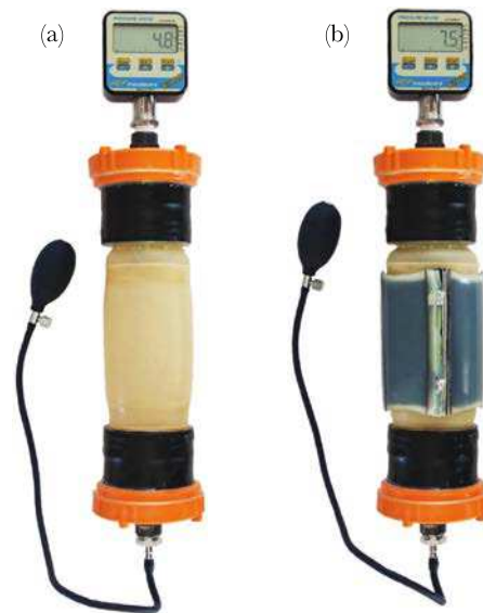
Fig. 3. Testing of the prototype dynamic bandages: air chamber that mimicked the compliance of a human limb, without (a) and with (b) the bandage.
