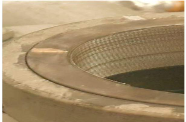
Figure 3. Nozzle with 150µm wire mesh.
