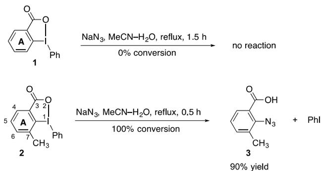
**Scheme 1.** Reactivity of 1-phenylbenziodoxolone **1** and 7-methyl-1-phenylbenziodoxolone **2** toward azide anion.
