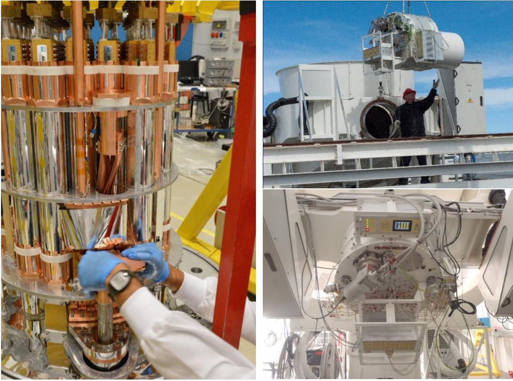
Figure 2: Left: TGI during the AIV phase. Right: TGI being installed in the QT2 focal plane on April 20th, 2016 (top), and a close view of the TGI with three pixels connected to the Back-End-Module (May 2016).
