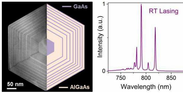
Cross-sectional image of GaAs/AlGaAs multi-quantum well (MQW) nanowire heterostructure (left) and room-temperature lasing spectrum from a GaAs/AlGaAs MQW nanowire (right).
