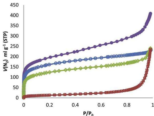
Fig. 2. N<sub>2</sub> adsorption isotherms for polymers P1-P4 obtained at 77 K.
